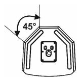
The rear side inclination, symmetrical, as shown in the upper picture, is 45°. KL15 can be used as a stage monitor in small contexts, in this case please consider the characteristic dispersion pattern presented above.
